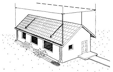
Area of sloped roof — (both sides) Length x width.
