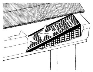
Gutter drain filter.
