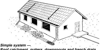
Roof catchment, gutters, downspouts and french drain.
