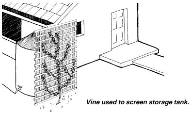
If storage is unsightly, it can be designed into the landscape by placing it in an unobtrusive place or hiding it with a structure, screen, and/or plants. Storage should be located close to the area of use and placed at an elevated level to take advantage of gravity flow. In all cases, cisterns should be placed a minimum of four to six feet away from the foundation in case of leaks. Ideally, on a sloped lot the storage area is located at the high end of the property to facilitate gravity flow.
