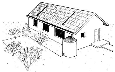
Complex water harvesting system with roof catchment, gutter, downspout, storage, & drip irrigation distribution system.
