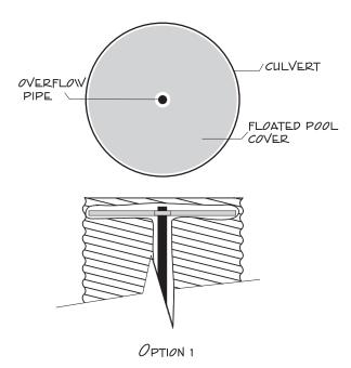
Option 1: Floating Cover - cut a piece of floated pool cover material to fit the inside diameter of the culvert. Place the cover inside the top of the culvert cutting a hole for the overflow pipe to pass through. The hole should be slightly larger than the overflow pipe to allow the cover to raise and lower easily, depending on the water level inside the cistern.
