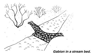
Gabions (a stationary grouping of large rocks encased in wire mesh) are widely used to contain water and reduce erosion. A trench is dug at least 12 inches deep across the wash, wire mesh is laid in the trench with the rocks to prevent undercutting.
