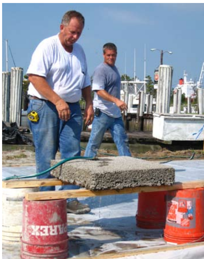
Contractors Thomas Homono and John Cobb demonstrate the permeability of pervious concrete at a Coastal Training Program event. (Photo courtesy, J. Pollack)
