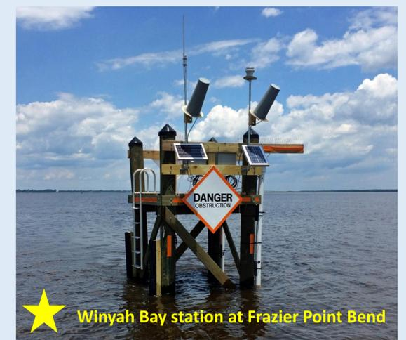
Measurements at this location are made at both surface and bottom since the central channel is deep and often stratified into two layers - fresher on the top, saltier on the bottom.
