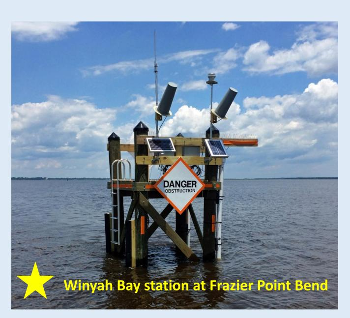
Measurements at this location are made at both surface and bottom since the central channel is deep and often stratified into two layers - fresher on the top, saltier on the bottom.
