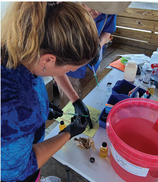
Volunteers learn how to use kits to measure the amount of dissolved oxygen in the water during a training workshop.
